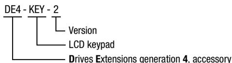
The optional LCD keypad DE4 4-KEY-2 can be used to configure drive controllers to your specific requirements.
